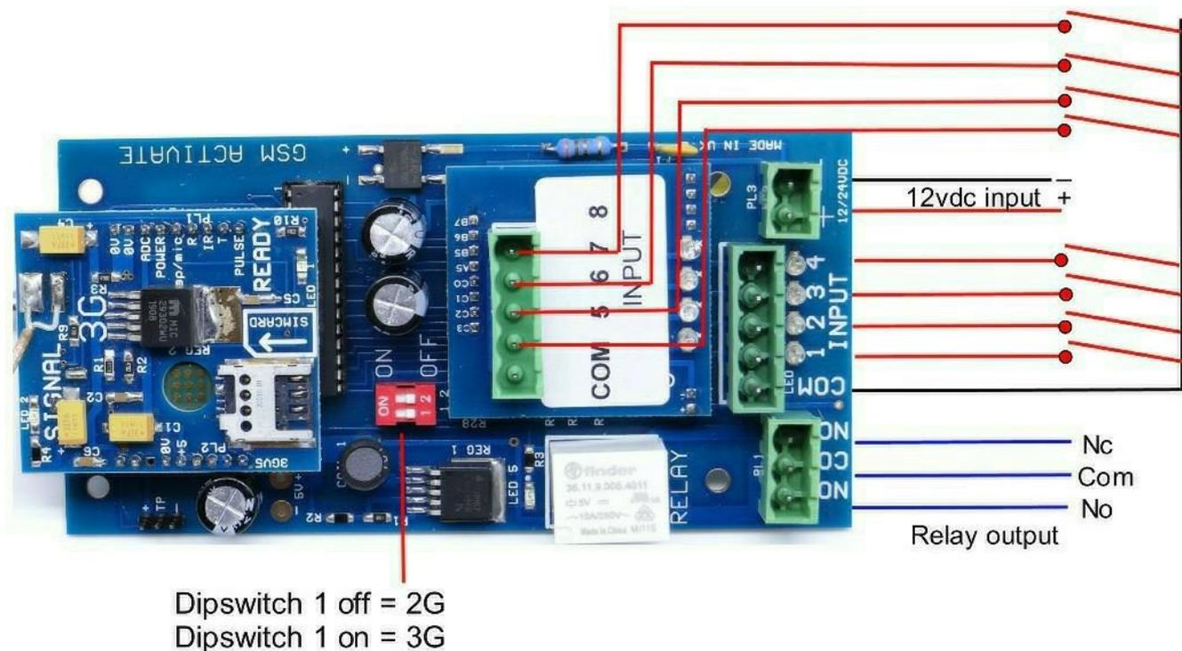
For alarm installations, please make sure you only supply a 9-24 volts DC from the battery terminals via the 2 amp fuse.
