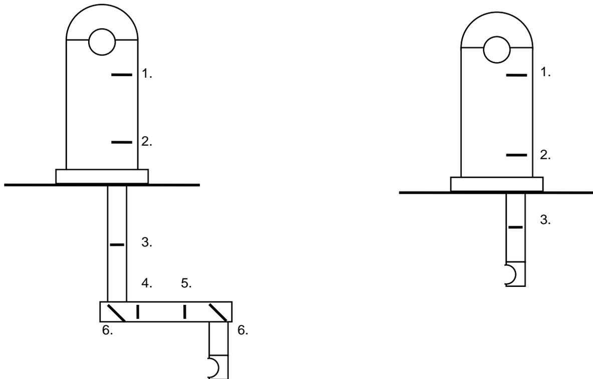
1. Upper part of the binnacle colum. Accessible by removing of compass.
