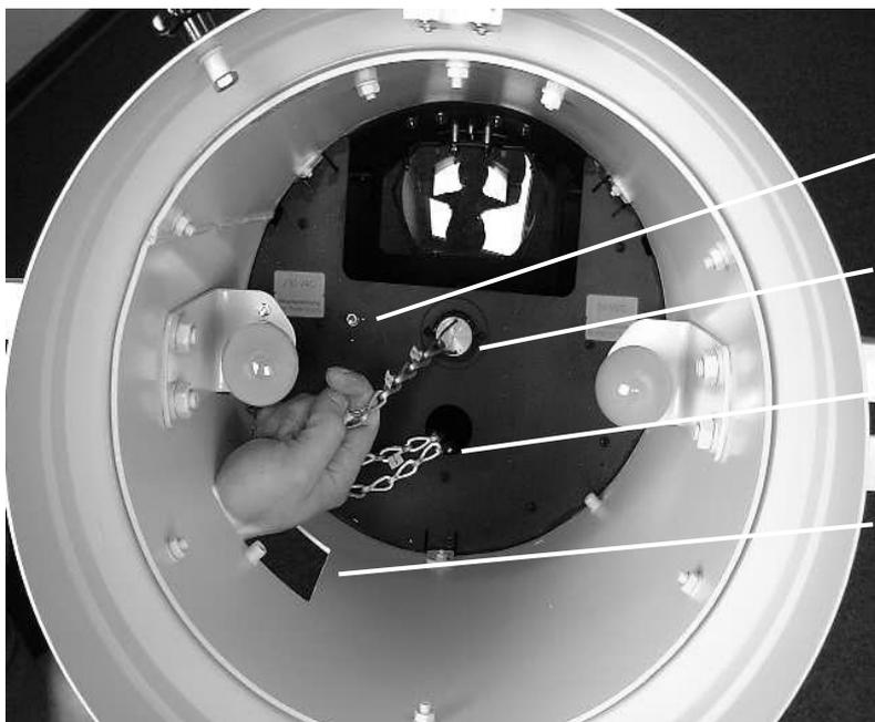
Screw to fix/loosen the chain
