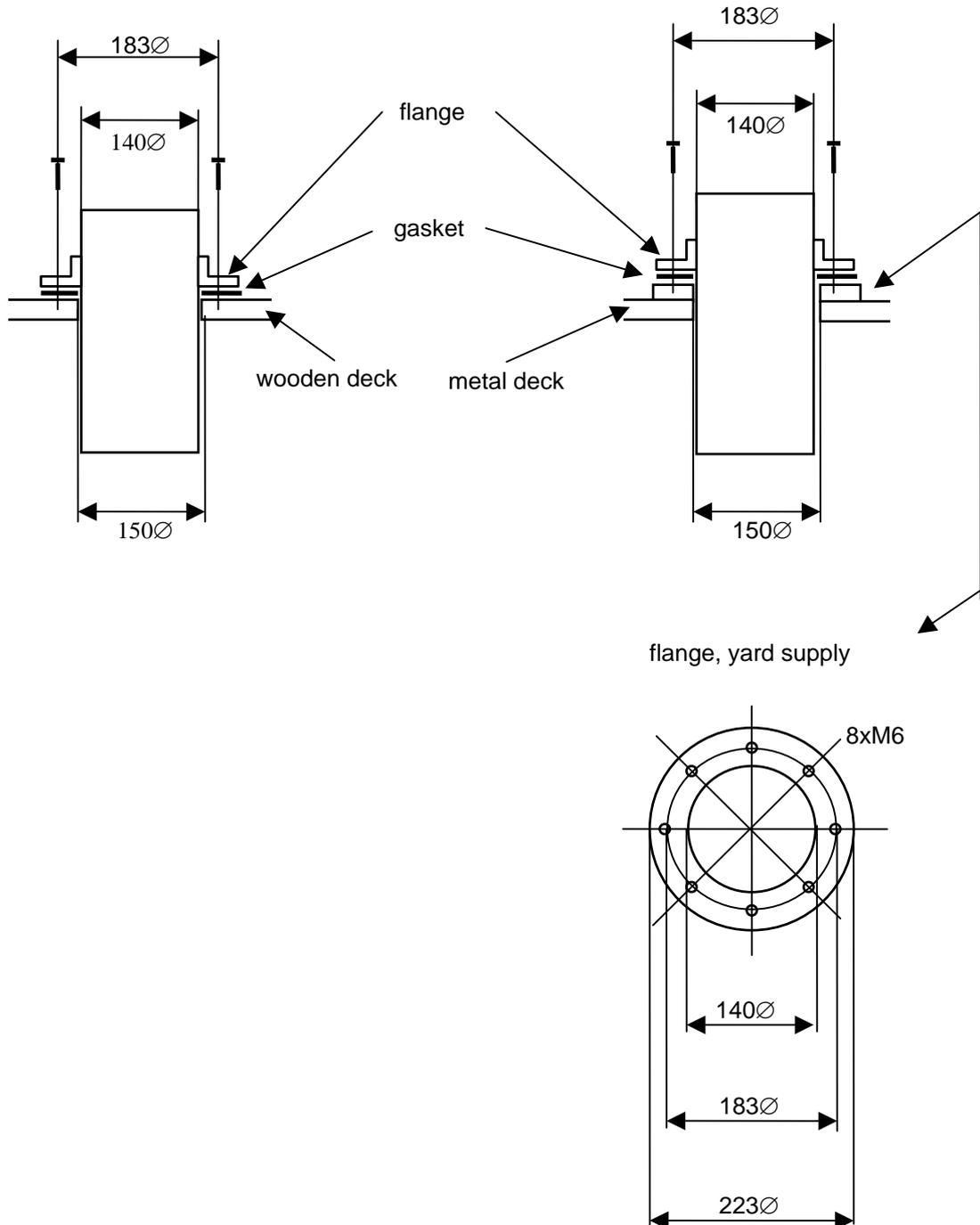
**Installation of Optical Arrangement (Reflection Tube)**
