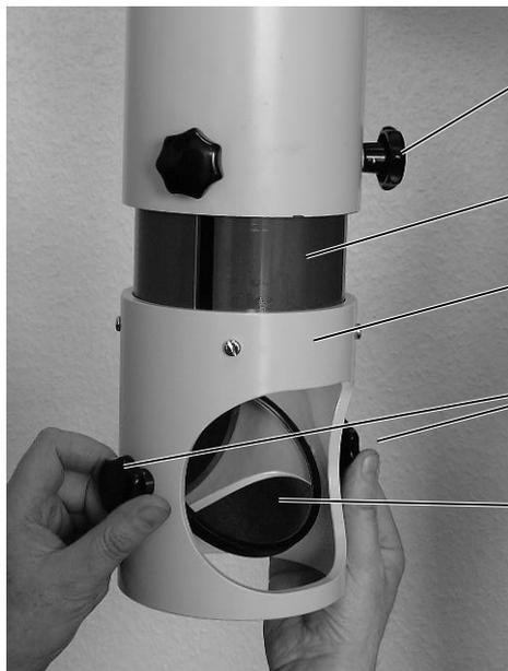
Arrest Knob to fix the extension tube
