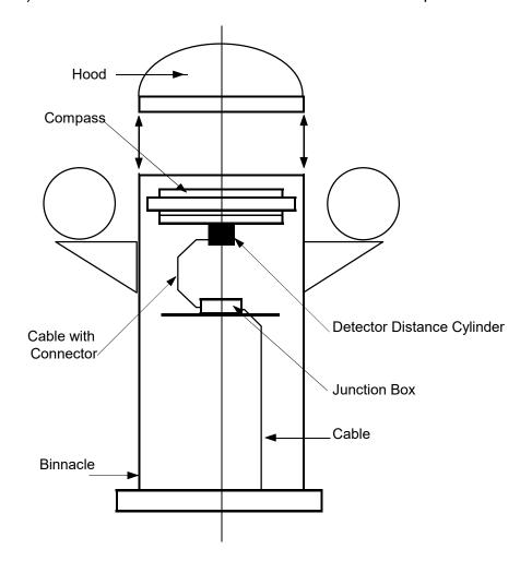
Attention: Make sure that detector cable does not impair free movement of compass gimbal and that cables do not obstruct visibility of reflection reading!
