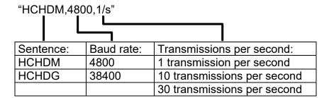
All transmissions are of 8 data bits, 1 stop bit and no parity.
