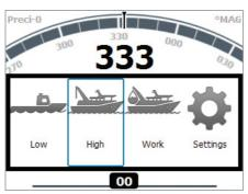
**Work mode:** Allows the autopilot system to be configured for optimal response in a specific situation, such as a fully laden vessel.
