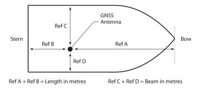
Figure 36 GNSS Antenna position
