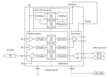
Figure 29 Input port schematic
