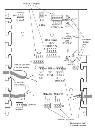
Figure 34 Junction box connections
