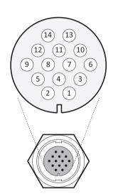
Figure 12 14-Way connector cable wiring connections
