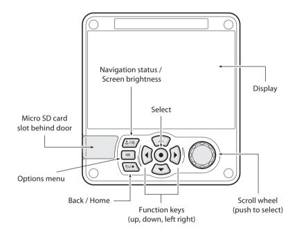
Figure 18 AIS Transceiver front panel
