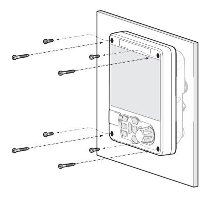
Figure 6 Panel mounting the AIS transceiver
