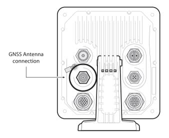
Figure 8 GNSS Antenna connection
