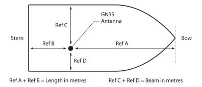
Figure 23 Vessel dimension measurement
