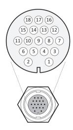
Figure 14 18-Way connector cable wiring connections
