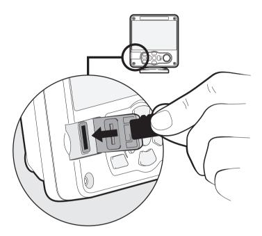
Figure 26 Micro SD card Socket
