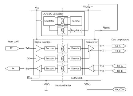
Figure 30 Data output port schematic
