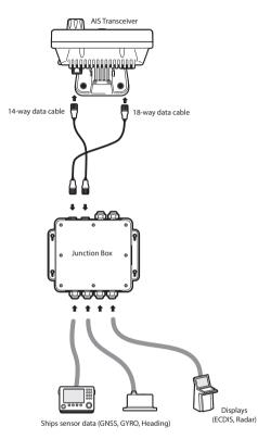
Figure 35 Connecting external equipment
