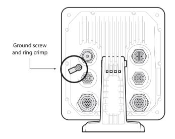
Figure 16 Grounding the AIS transceiver
