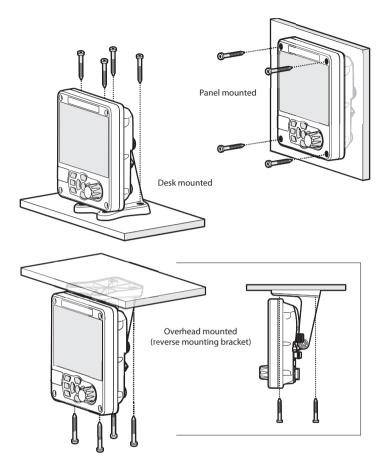
Figure 4 Mounting the AIS transceiver
