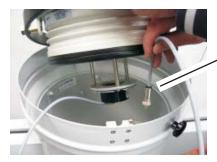
When lifting the compass watch & unplug detector cable, if any!
