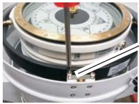
Open fixture of compass suspension
