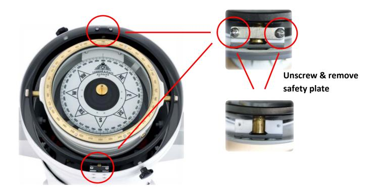
Reassembling will be done in reverse order. Take attention of ahead marking on compass bowl! Compass may swing within its balance ring, take care of your fingers! Make sure that cables do not obscure reflection sight nor impair free swing of the compass
