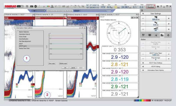
The CP60 can measure current speed and direction in up to 5 layers in the water column. The depth of the layers can be easily set by the user as well as the number of layers (between 1-5) (1). When used together with an ES80 echosounder (as in the picture above), the current profiling will show as a tab where the user normally can select between frequencies/transducers (2).
