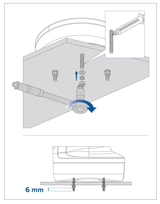
13. Ensure all 4 sets of nuts and washers are used to secure the pedestal to the mounting platform. There should be no more than 6 mm of excess stud below the nut. Cut-off any excess stud.
