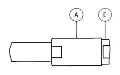
Push body A over clamp ring B. Screw back nut A onto body C and tighten with spanner (torque 19 Nm). Keep cable to prevent rotation with back nut A.
