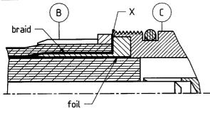
Open carefully jacket. Press foil onto dielectric. Push sleeve of body C under braid and over foil. Slide clamp ring B to body C. Remove protruding braid flush with clamp ring B at X.
