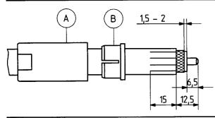
Slide body A and clamp ring B over cable. Prepare cable according to diagram. Remove braid and foil 1,5mm - 2mm. Trim edge on centre conductor with file. Cut jacket 4-6 times lengthwise 15mm CAUTION: Do not damage braid. Important: Clean centre conductor with sand paper. All dielectric rests must be removed.
