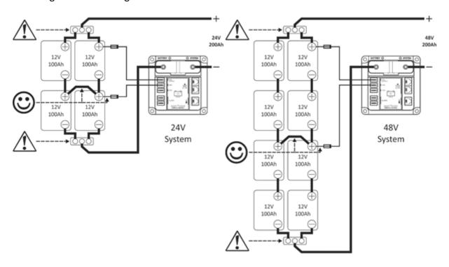
The above images are also indicating that busbars are being used to respectively join all positive and all negative battery cables. Besides this, all positive and negative battery cables that are wired to these busbars need to be of equal length. These precautions are made to avoid any imbalance between the different series strings, to ultimately improve the overall accuracy of the midpoint voltage measurement.
