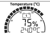
Shows the battery temperature when a temperature sensor is connected to the Expert Modular. The default temperature unit is °C, but it can be set to °F as well in Function F10.3.
