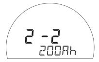
The default battery capacity value is 200Ah. This can be changed by pressing the left or right arrow keys until the desired value is reached. The standard battery capacity value is based on a discharge rate of 20 hours. When your battery capacity is rated at a different discharge rate, please change this in Function F1.2 (see chapter 6.1) afterwards. Once the selection has been made, press the MENU key for 3 seconds to finalize the Setup wizard.
