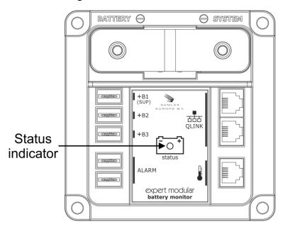
The status indicator has multiple operating modes, distinguished each by colour or flash interval. Please see the table below for an overview of the operating modes:
