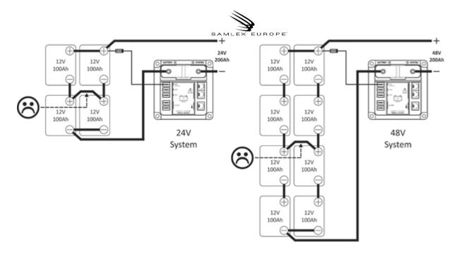
The reason for this is that through the interconnected midpoints, one bad battery in a series string can damage all other batteries if not being monitored correctly. However, when decent midpoint voltage measurement has been applied and an alarm is triggered when the voltage difference is too large, the midpoints of the series strings are allowed to be interconnected. This will result in the following connection diagrams:
