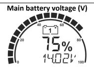
Shows the voltage of the main battery bank connected to the +B1 input.
