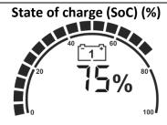
The SoC is the most important battery parameter. It shows exactly how much charge is left in the battery. This value is compensated for all known battery variables (age, charge/discharge current, temperature etc.). 100% represents a fully charged battery, while 0% represents a completely flat battery. Typically, you should recharge a lead based battery when the SoC has dropped below 50%. For a lithium based battery, this level can be lower.
