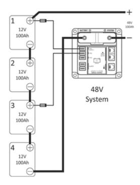
Please note that when using the +B2 input for midpoint voltage measurement, you should set Function F2.0 to 'MIDPNT'. You can also configure the +B3 input for midpoint voltage measurement, but only one of these two inputs can be used at the same time for this purpose.
