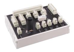
The MS431 board is the base unit for connection of the MS421B BNWAS.
