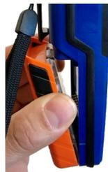
3. Squeeze in the black finger grips on either side of the battery to lock the battery into place
