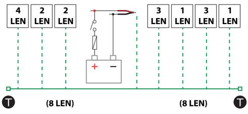
Note: Do not connect the NMEA 2000<sup>®</sup> power cable to the same terminals as the engine start batteries, autopilot computer, bow thruster or other high-current devices.
