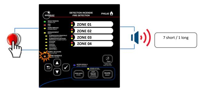
This audible sequence informs that it's necessary to evacuate the ship. This sequence is constinutly repeated as long as the general alarm input is active. The general alarm indicator lights up to indicate that the general alarm sequence is launched.
