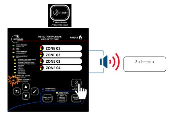
A long press (>3 seconds) on the "acknowledgement" bouton allows to launch an audible and visible test:
