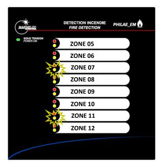
In the disablement menu, the yellow zone fault LED illuminates to indicate that corresponding zone is disabled. In the above example, zones 4, 7 and 11 are disabled.
