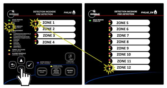
If you press the down arrow when the cursor is placed on the last zone, the cursor will be place on siren fault indicator. To disable/enable the current zone/output siren, it's necessary to press "validation" button. After this action, the cursor is automatically placed on the next zone/output siren.
