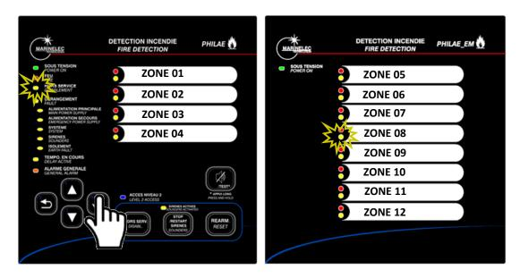
When the cursor selection shows the correct zone (yellow LED flashing), press "validation" button to change the zone status. In the example above, zone 8 will turn from Enabled to Disabled.
