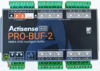
Two OPTO-isolated inputs and twelve ISO-Drive<sup>™</sup>isolated outputs. Offering device protection and excellent flexibility, all in one product.
