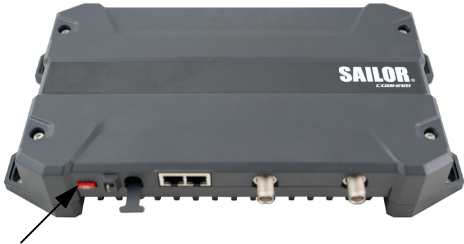
Figure 3: Replacing the fuse in the SAILOR 7226 VHF Transceiver Unit
