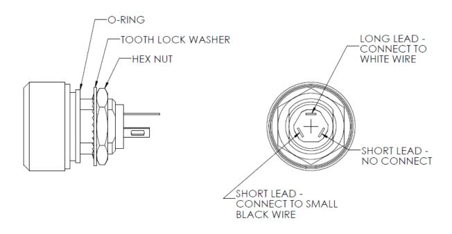
FOR NON-DIMMING OPERATION SHORT BOTH SMALL WIRES TOGETHER
